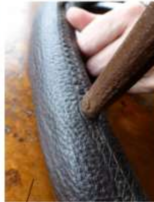
Stitched circular leather handrail.
